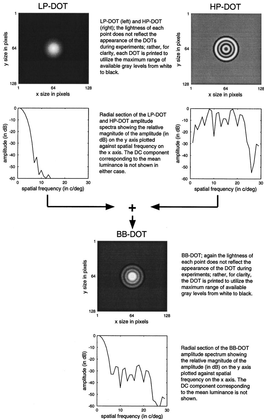
Fig. 5. Process of stimulus generation of the BB-DOTs shown in both the space and the spatial-frequency domain. Note that all three types of DOTs are printed with use of the maximally available range of gray levels and thus have much higher contrast than the ones actually displayed during the experiments. Further, the HP-DOT was appropriately scaled before being added to the LP-DOT; see the text for details.
